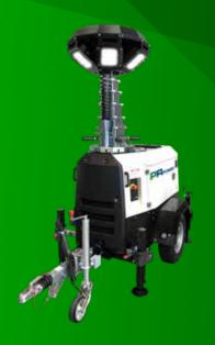
The PR-ECO 360° LED Mobile Lighting Tower units utilise highly efficient LED lamps mounted atop an 8.5m vertical, hydraulic mast with a 48vDC extra low voltage lighting system and the Automatic Mast Operating Safety System (AMOSS) for added safety and environmental sustainability.
