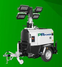
The PR-ECO LED (4 x 320W) Mobile Lighting Tower units utilise highly efficient LED lamps mounted atop an 8.5m vertical, hydraulic mast with a 48vDC extra low voltage lighting system and the Automatic Mast Operating Safety System (AMOSS) for added safety and environmental sustainability.
