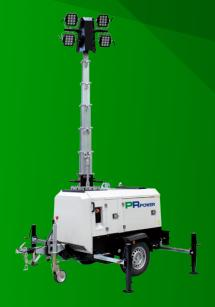
The X-HYBRID LED Mobile Lighting Tower units utilise highly efficient LED lamps mounted atop an 8.5m vertical, hydraulic mast with a 48vDC extra low voltage lighting system.
